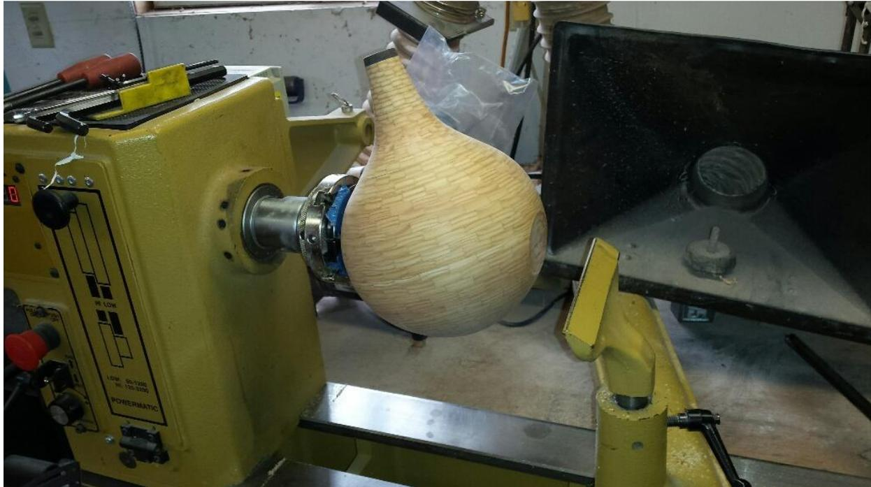
It looks like I stopped taking photos at this point, that is the last one I have! The teapot was reversed again into a small vacuum chuck so that the hole could be trimmed and finished with CA glue. The final finish was applied at this point on the lathe sometimes rotating and sometimes stationary.
