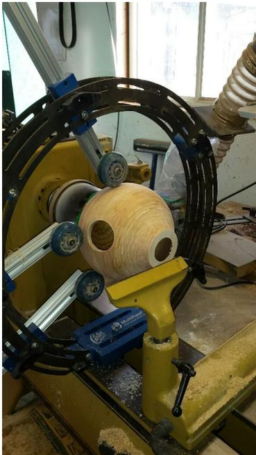
The spout was already assembled on my small lathe and hollowed, here it is glued in place, then turned and finished with CA glue:-
