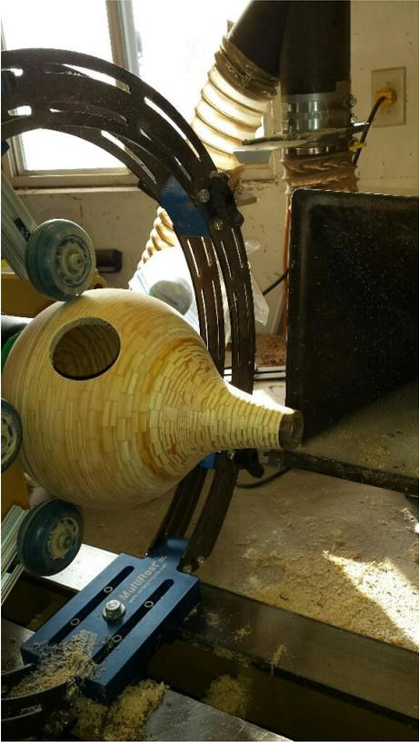
The teapot is then mounted in a 4 jaw chuck using the lid hole and the bottom is turned. This is where you realize you should have left the walls a little thicker....
