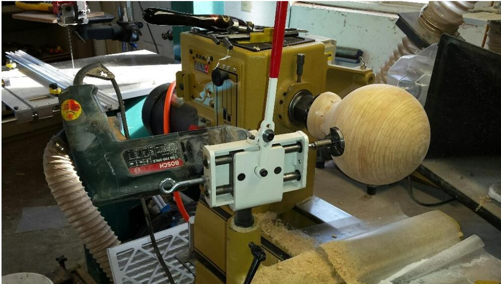
The teapot was then mounted in a vacuum chuck in order to take off the other face plate and finish the surface ready to mount the spout:-
